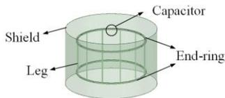
Fig. 3. The model of the high pass birdcage coil.
