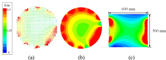
Fig. 4. (a) The vector H field and (b) The complex magnitude of H field in the transverse cross-section of the birdcage coil. (c) The complex magnitude of H field in the longitudinal cross-section of the birdcage coil. The longitudinal and the transverse cross-section both cross the center of the coil.
