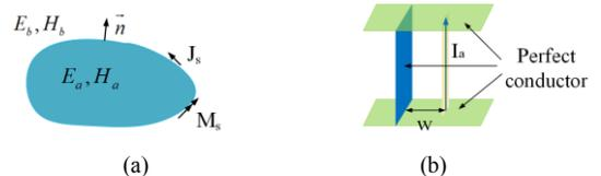
Fig. 1. (a) A diagram illustrating the equivalence principle. (b) A simple active Huygens' metasurface element with a perfect conductor.
