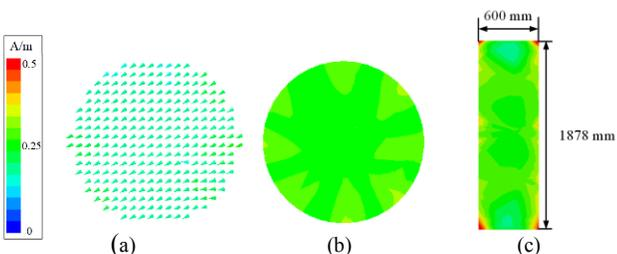
Fig. 5. (a) The vector H field and (b) The complex magnitude of H field in the transverse cross-section of the Huygens' box. (c) The complex magnitude of H field in the longitudinal cross-section of the Huygens' box. The longitudinal and the transverse cross-section both cross the center of the Huygens' box.
