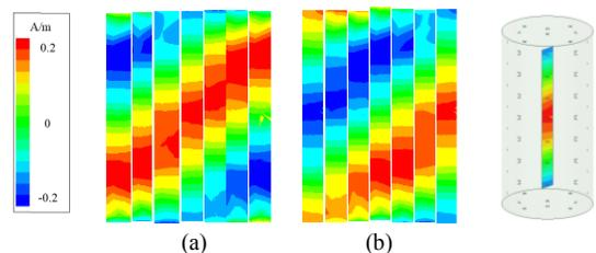
Fig. 6. (a) The x and (b) The y component of H field at  $0^\circ, 30^\circ, 60^\circ, 90^\circ, 120^\circ, 150^\circ, 180^\circ$  at the longitudinal cross-section of the Huygens' Box.
